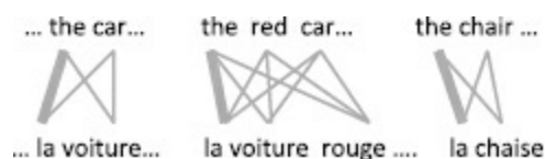
Figure 14 After the first iteration, the algorithm identifies the link between “la” and “the” as being the most likely, based on their frequency in the source language and in the target language. These links are strengthened (shown in bold) to the detriment of other links
