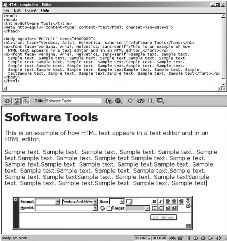
Fig. 3 HTML document viewed in a text editor and the same document viewed in an HTML editor in document layout mode
