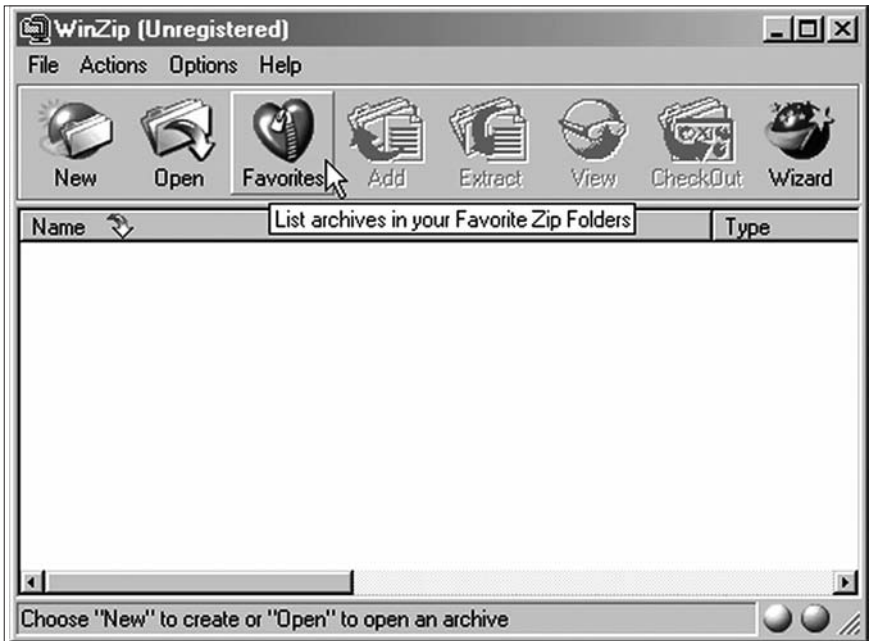
Fig. 1 WinZip® user interface displaying the tool tip text for Favorites and quick information in the status bar
