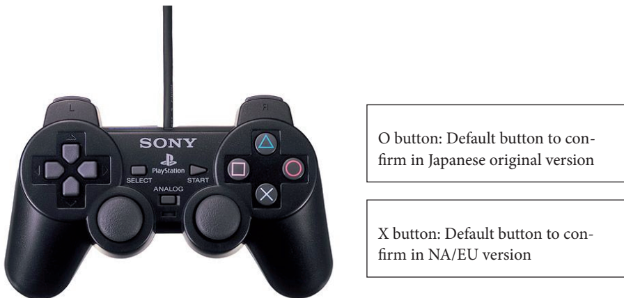
Figure 3.1 Differences in button mapping in PlayStation® 2 Controller
