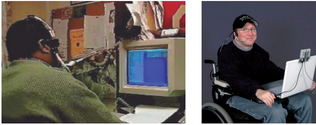
Figure 7.2 Head mouse 106 and sip-and-puff switch 107
